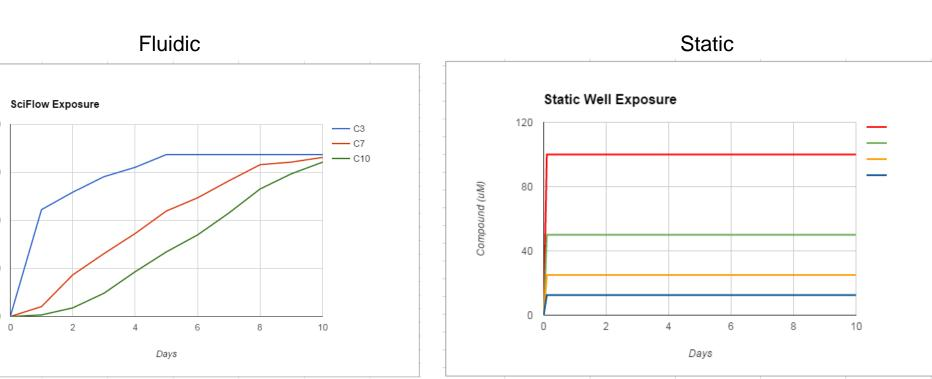
In an acellular scenario (A), SciFlow (left) dosing creates gradients of compound concentrations over time. The concentration of compound increases in each well until the equilibrium concentration is reached, and then that concentration is maintained for the duration of the experiment. Wells at different distances from the source well have very different concentration exposure profiles. Static plates (right) are at a fixed concentration, which only varies due to cellular metabolism.
