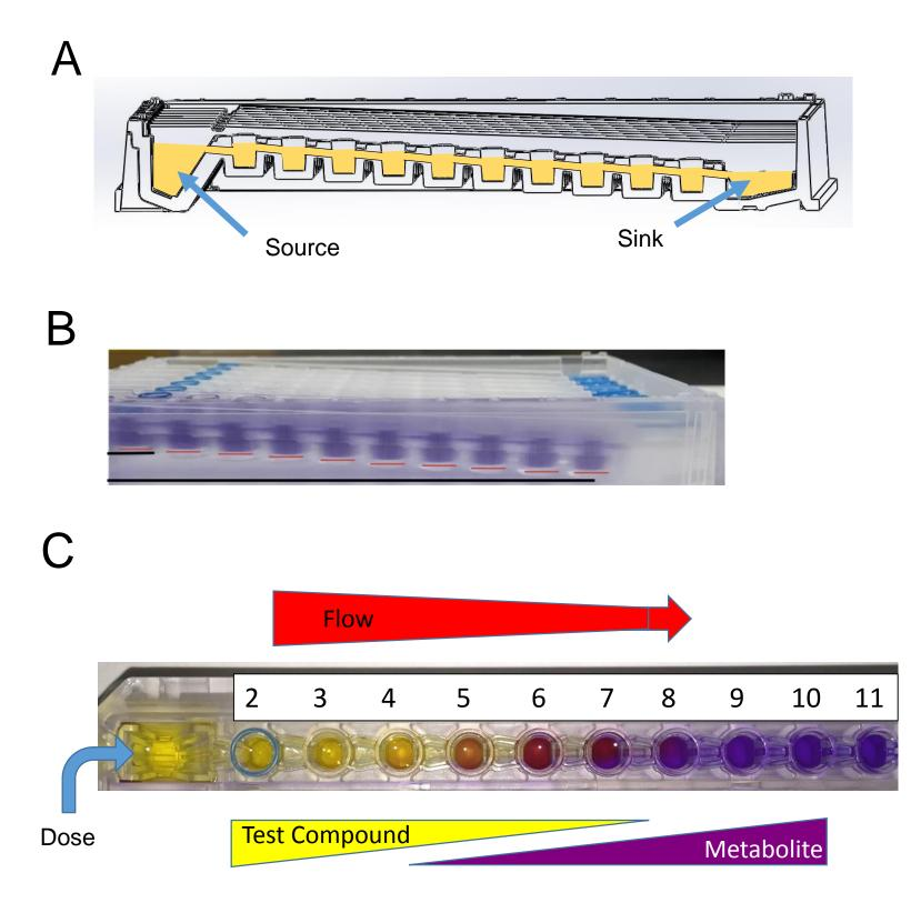
Panel A shows a schematic side view of SciFlow with the source and sink wells identified 0.5mm decrease in height for each well bottom. Panel B is a picture of SciFlow, with purple liquid filling one row to highlight the 0.5mm decrease in Z-height (height of well bottom) across the plate. Panel C is a top down view of one SciFlow row highlighting the dual gradients of decreasing parent compound and increasing metabolite down the row.
